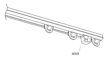
Smart application of the spring stop 4003, in a punch. The last glider 6009 functions as an end stop, since it is locked between the 4003 and the end of the slot, or between the 4003 and the wall.
