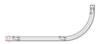
when mounting a curved rail, place a ceiling mounting clamp before as well as after the curve
