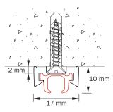
ceiling mounting 2400 with ceiling clip 2450 and sunken head screw, max. screw diameter 3,5 mm.
