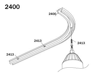
application of the Torx screws during ceiling mounting of a pre-punched 2400 rail
